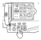
You can conduct an image search (P31) by holding down the ◀◀ button in the shooting pause mode. Do not hold down the ◀◀ button when conducting a rec check.
